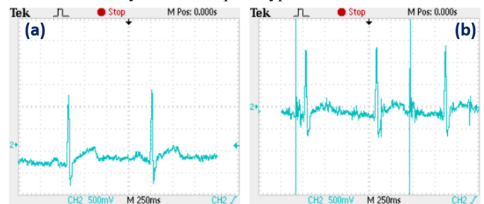
Fig. 5 Prototype result with (a) finger movement (b) the subject walking.
