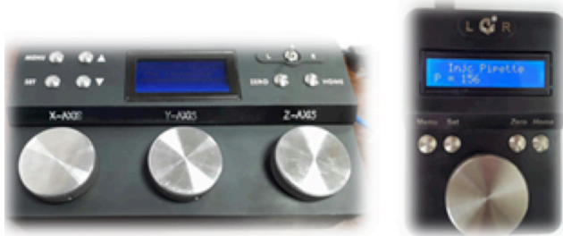
Fig. 4. Overview of Controlling Devices of Micromanipulation and Microinjection. (a) Micromanipulator Controller (b) Microinjector Controller
